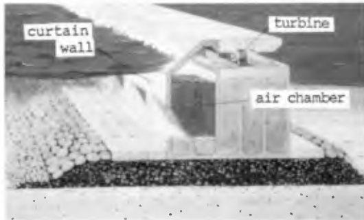
Fig.1 Wave Power Extracting Caisson Breakwater
