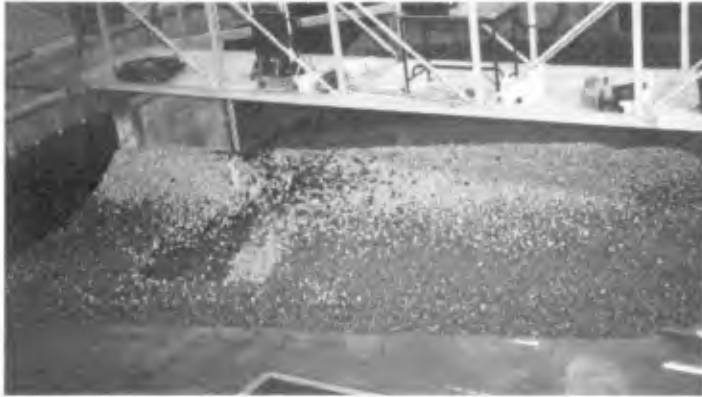
Fig 11. Example of the breakwater after longshore transport tests in oblique waves.
