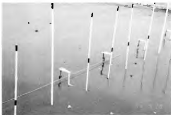
Photo 1 Run-up meter and stick array.
