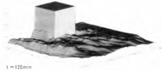
Fig.13 Bird's eye view of measured bottom change (Square-I, \theta=0^\circ , T=1.0\text{s} , H=10.0\text{cm} , t=120\text{min} )
