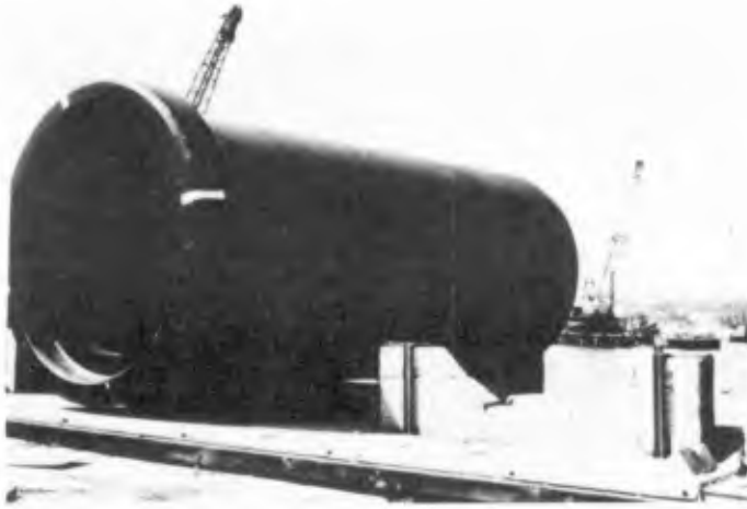
COAL-TAR EPOXY FINISH ON PIPE
